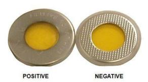
EQ-CR2016-Kapton-2s is special CR-2016 coin cell casing with two sides of 10mm Kapton windows to achieve a full penetration of in-situ neutron diffraction This design creates the possiblity to analysis of battery material phase variations during charging and discharging.
