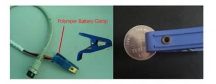
CT-4000 Multi Range mA Battery Testing System, characterized with 0.05% FS accuracy and down to  $\mu$ A capability, enables users to perform DCIR tests, dQ/dV and other basic tests on three-electrode system. It mainly focuses on battery research & development institutions and universities.
