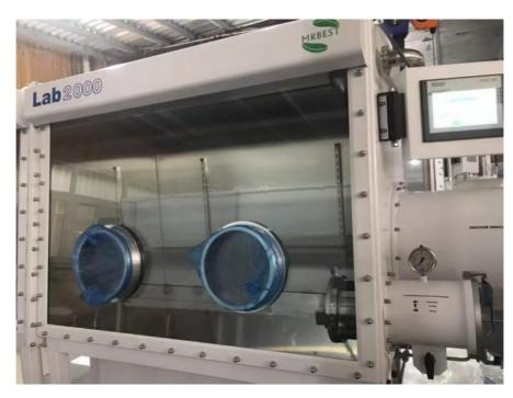
Lab 2000: Standard features of this system include a large main antechamber, a rotary vane vacuum pump and a microcontroller with operation panel.
