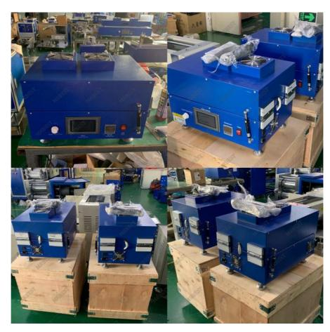
MR-TMH250 is a compact film tape casting machine with vacuum chuck, which widely used in all kinds film coating research, like ceramic films, crystal films, lithium battery electrode coating, etc. It is designed with top cover heating, the heating temperature up to 150 adjustable and digital display.
