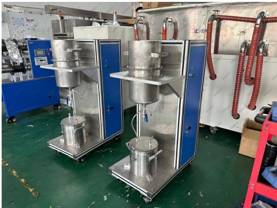
MR-GL-2-5L is used for battery slurry iron removing and filtering.
