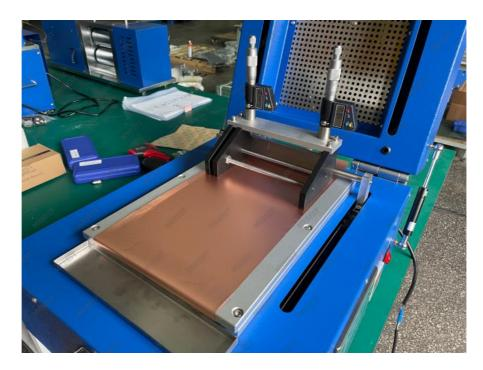
MR-TMH250 is a compact film tape casting machine with vacuum chuck, which widely used in all kinds film coating research, like ceramic films, crystal films, lithium battery electrode coating, etc. It is designed with top cover heating, the heating temperature up to 200 adjustable and digital display.
