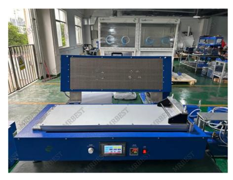
MR-TMH800 is a large desktop film tape casting machine with vacuum chuck, which widely used in all kinds film coating research, like ceramic films, crystal films, lithium battery electrode coating, etc. It is designed with top cover heating, the heating temperature up to 150 adjustable and digital display. The coating speed, coating stroke length, coating thickness adjustable. 800mm coating length makes it perfect for cylindrical cell electrode coating.
