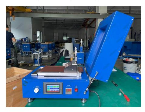
MR-TMH250 is a compact film tape casting machine with vacuum chuck, which widely used in all kinds film coating research, like ceramic films, crystal films, lithium battery electrode coating, etc. It is designed with top cover heating, the heating temperature up to 150 adjustable and digital display.
