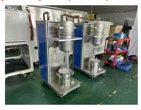
MR-GL-2-5L is used for battery slurry iron removing and filtering.
