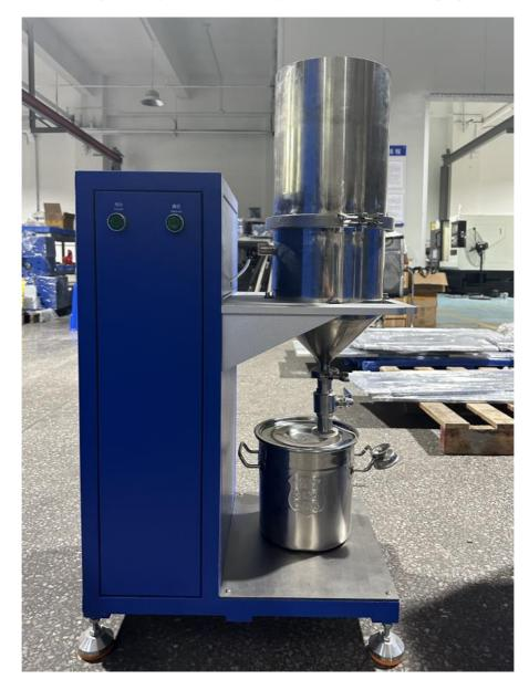
MR-GL-2-2L is used for battery slurry iron removing and filtering.
