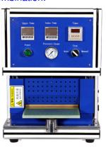
\* B. Vacuum Sealing Machine (for pre-sealing in glove box after injection of electrolyte)
